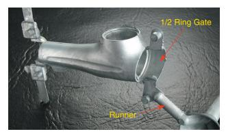
The overflows are positioned on the thin section end of the elbow furthest from the inlet gating. They also use a 1/2 ring geometry (with side tabs) on the thin end to avoid trim blemishes on the visible body of the elbow.
