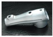
The as cast elbow housing
