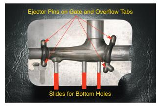
Ejector pin placement
